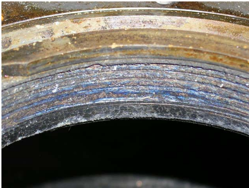
Photo No. 13 Interstage airseal detail, approximate 9:00 position.
