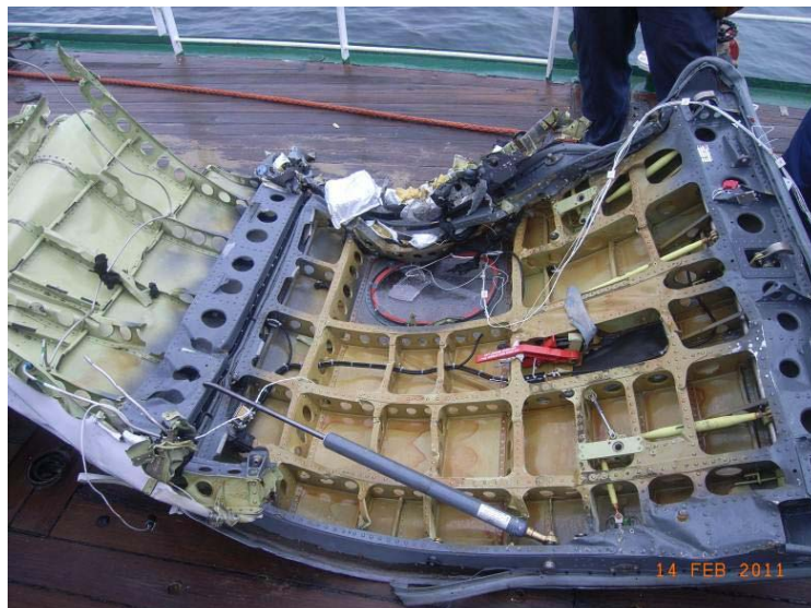
Figure 11. Cargo door with shoot bolt.
