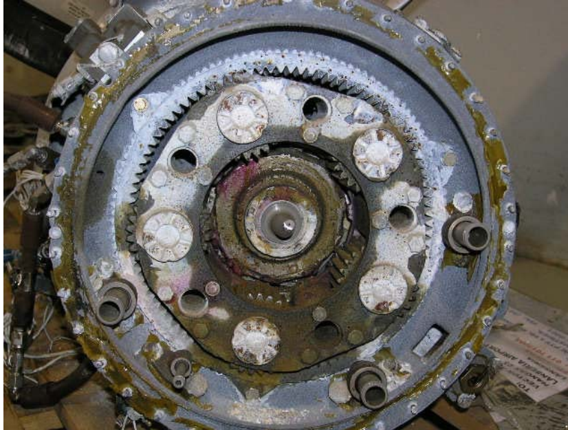
Photo No. 19 Reduction gearbox 2nd stage gearing.
