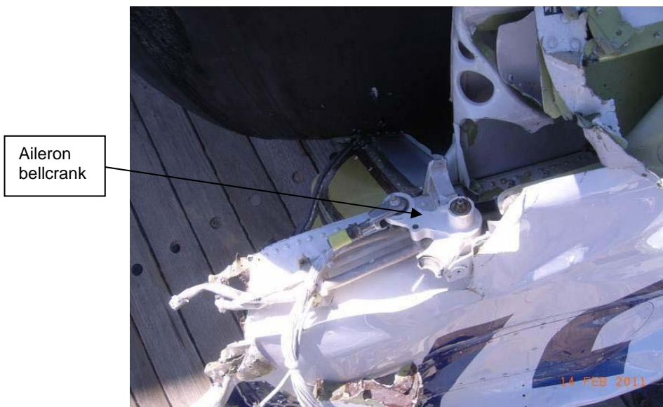
Figure 9. The left-hand outer aileron bell crank.
