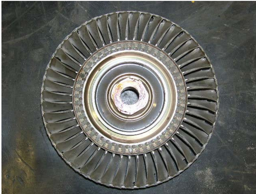
Photo No. 10 1st stage power turbine, upstream side.
