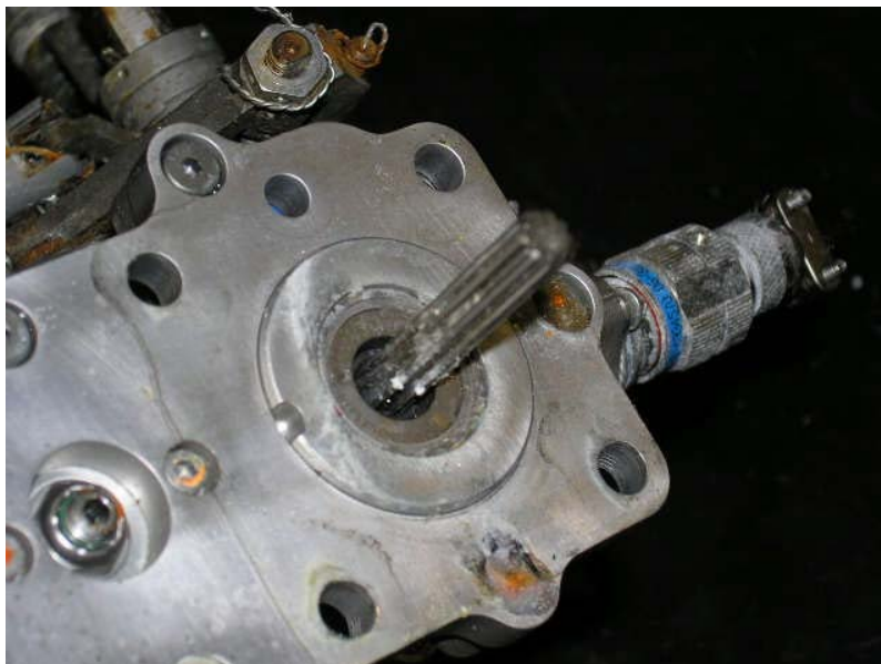
Photo No. 22 Fuel control unit governor drive shaft.
