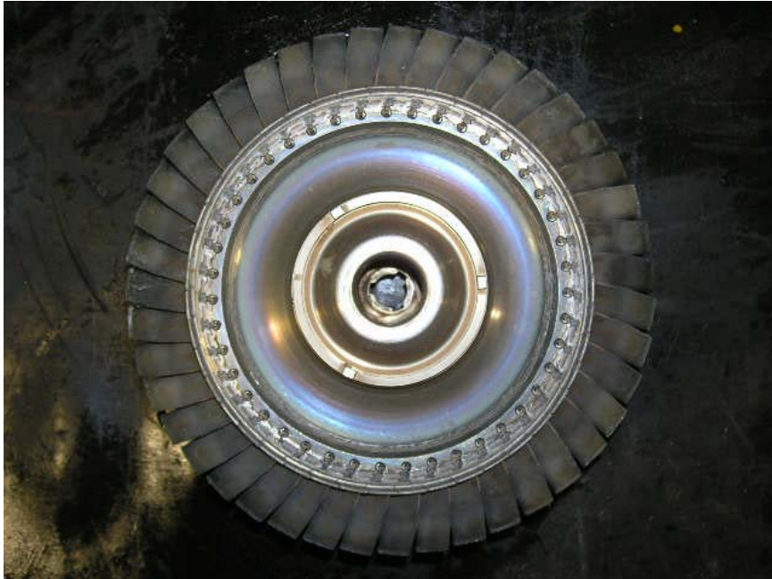
Photo No. 8 Compressor turbine, downstream side.
