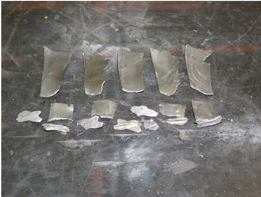
Photo No. 17 Recovered 2nd stage power turbine blades.
