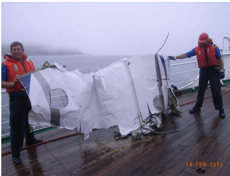
Figure 13. Top part of cargo area, fuselage section.
