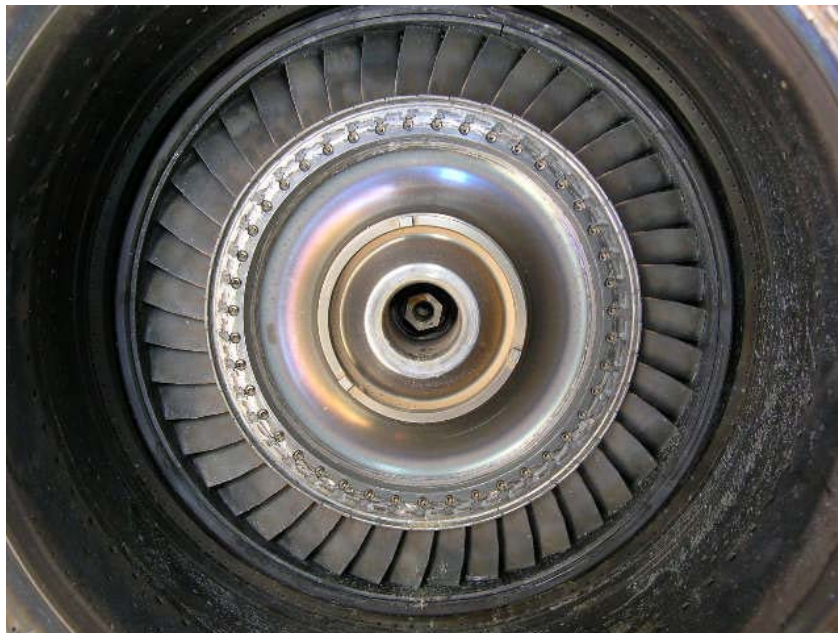
Photo No. 7 Compressor turbine, in-situ.
